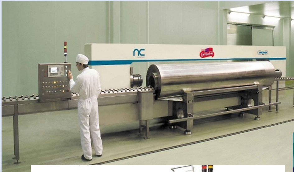
QFP 320L-400 High Pressure Seafood Processing System
