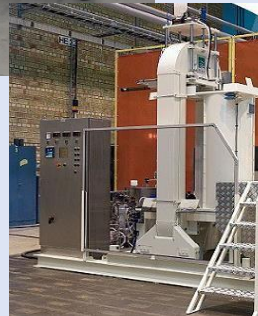
QFP 320L-400 High Pressure Seafood Processing System
