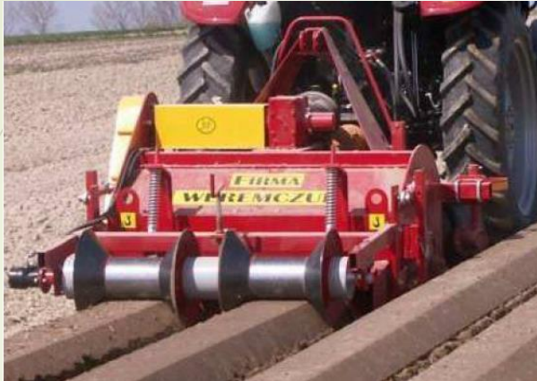
Ridge former with cutter "AUR" and rollers
