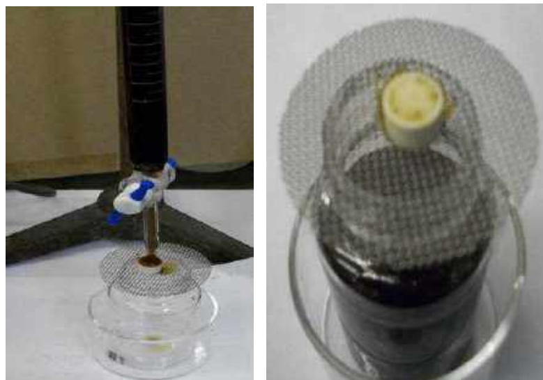
Fig. 2. Experimental set up for retrieving magnetotactic bacteria from molasses-based animal feed (A); appearance of colored magnetotactic bacteria on the surface of Neodimium magnet (B)
